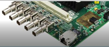
The Media Server IP (MS-IP) is a digital media server capable to produce multiplexed signals over one or multiple IP outputs 24 hours a day.
