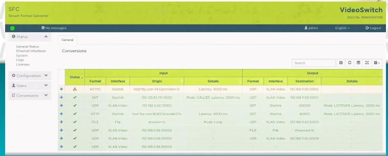
The SFC (Stream Format Converter) is an OTT format converter with one or more IP inputs and outputs, capable of converting live signal streams or files from one OTT format to any other.
